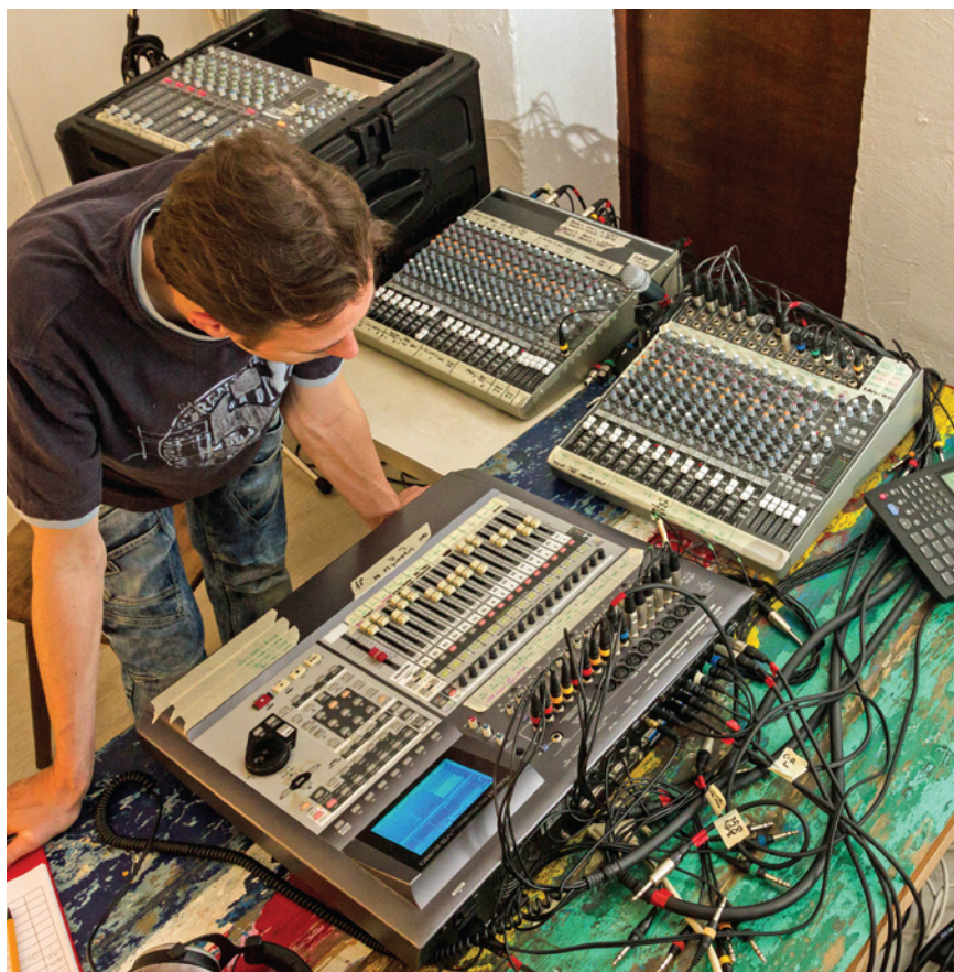
Frequent band line-up changes between numbers meant a great deal of rerouting and replugging. To avoid confusion and wasted session time, Mike labelled all the main control-room devices extensively with masking tape, as you can see here.
